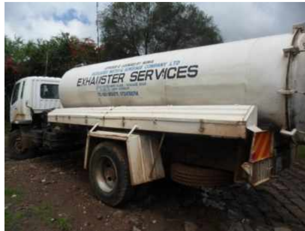
Figure 6: Exhauster from Oloolaiser Water and Sewerage Company
